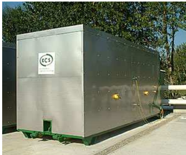
Figure 108: The stainless Steel Containerized Vessel employed for Composting
