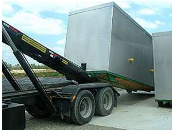
Figure 109: The roll-off truck is used to move and unload the vessels.
