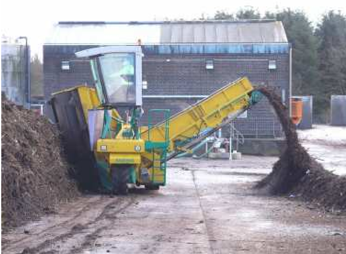
Figure 59: Agitation of the Curing Windrows through an Extended Bed Turner
